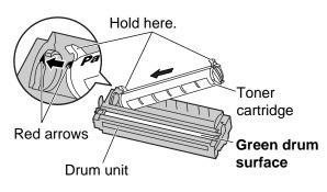
Slide the tab of the toner cartridge into the slot of the drum unit.
